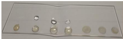
10 \mu\text{L} of DNA ( 1\mu\text{g}/\mu\text{L} ) in pure water left to dry on a \text{CaF}_2 microscope slide
